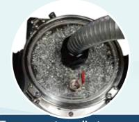
Transparent acrylic top cover provides a clear view in the filter bucket Suction hose is wrapped at the end to prevent clogging
